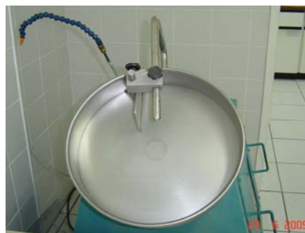
Figure 2: Rotation dish granulator used for grain preparation of clay and urea.
