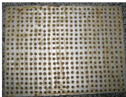
Figure 1: Perforated plates used for grains preparation of clay and urea.
